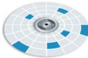
Figure 5.12 - How a file is stored in different places of a disk
