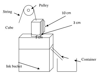
The above set up was prepared to fill some ink bottles equally. There is a cube of metal with the length, breath and the height are 5 cm, 3 cm and 10 cm. When the cube is immersed in the ink a volume of ink is displaced out to the ink bucket.
