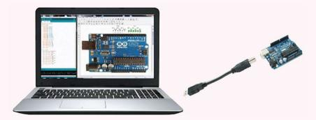
The cable connecting the Arduino Board to the computer has USB at one end and miniUSB at the other. The USB is connected to the computer and the miniUSB is connected to the Arduino Board.
