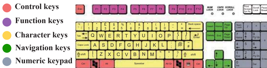
Figure 4.1 Key arrangement on a typical keyboard
