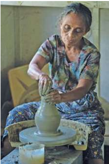
Fig. 1.11 Making clay pots using pottor's wheel
