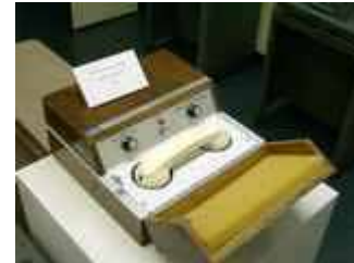
Anderson Jacobson ADC 260 acoustic coupler 1963, from SDCM
