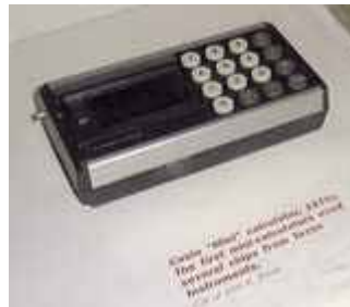
early transistor calculators - Casio "Mini" used chips from TI (left); TI SR-10 calculator showing circuit in transparent case, used a single chip 1972, from Smithsonian NMAH
