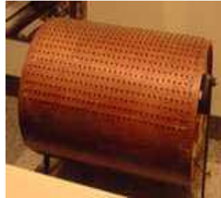
magnetic drum memory of the Atanasoff-Berry Computer 1939, from Smithsonian NMAH
