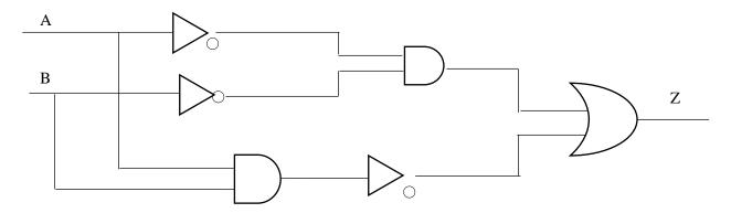
Write the output of Z in the above circuit.
